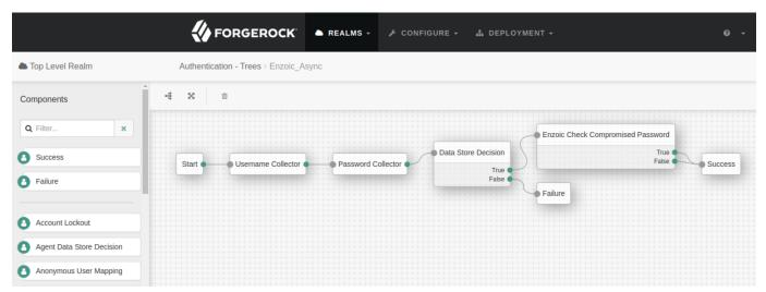
The Enzoic Sync Auth Tree will check if the password is compromised using the Enzoic API. This tree then waits for a response from Enzoic before proceeding. If the password is compromised, the user will not able to login.
